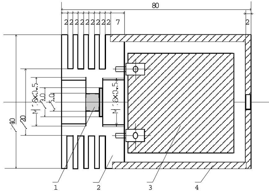
Fig.2. Mechanical structure of the laser irradiator: 1 - laser diode, 2 - cooling radiator, 3 - electronic supply driver, 4 - protective plastic cylinder
