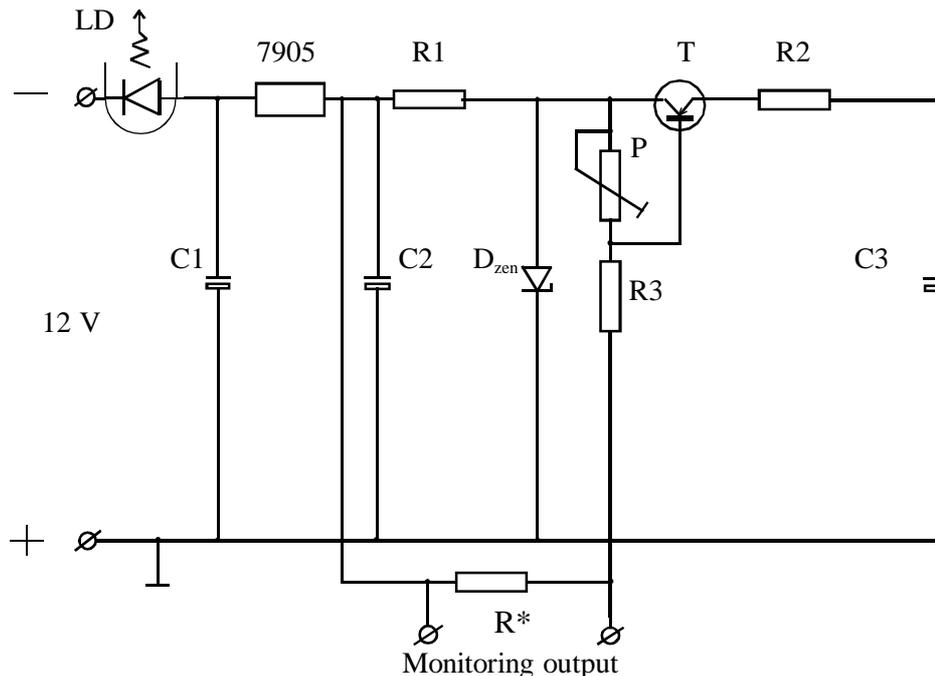
Fig.1. Electronic circuit for diode power supply:  $D_{zen}$  – zener diode, selected 5V
