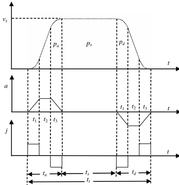
Fig. 1. S-curve profile with symmetrical acceleration and deceleration periods
