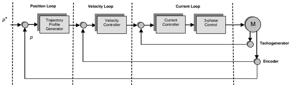
Fig. 2. A block diagram of 3-loop control scheme of an AC motor
