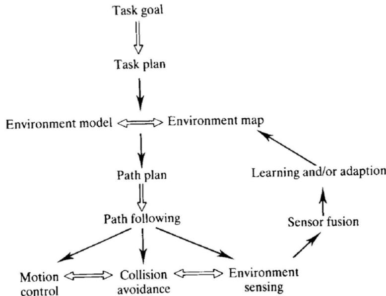
Fig. 2. Mobile robot control hierarchy, showing information flow
