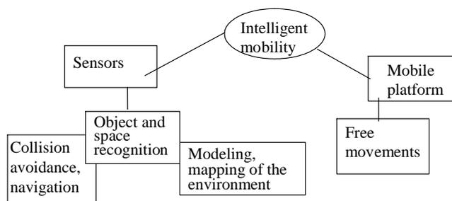
Fig. 1. Components supporting intelligent mobility
