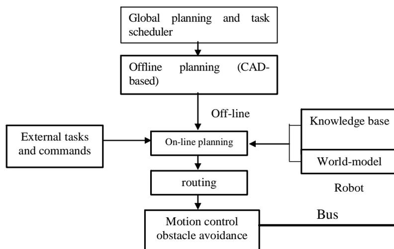
Fig. 4. Task planning of mobile robots
